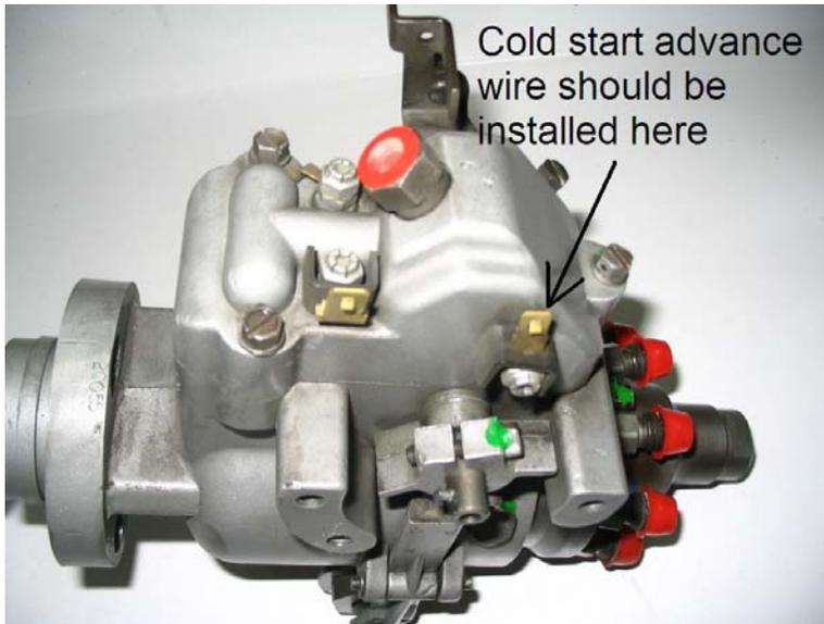
2) You should also have the pump properly timed. Please refer to the manufacturers timing information for complete timing instructions. Most 6.9 and 7.3L applications, when properly timed, have the timing mark advanced (toward the drivers side of the vehicle) approximately 1/8 inch off the engine timing mark.
